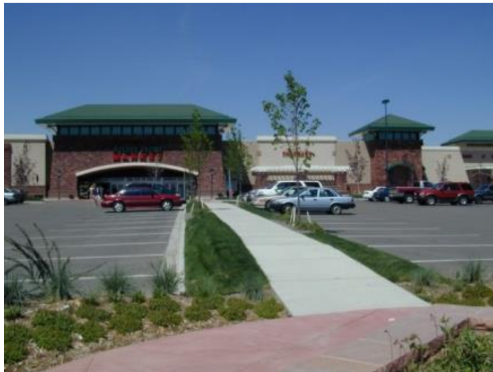
Figure 11.09-A: This photograph illustrates how a sidewalk connecting the public sidewalk to the business can be integrated into the required landscaping.
